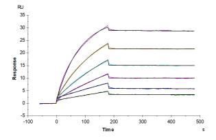
Biotinylated Human CD20 VLP captured on CM5 Chip via streptavidin can bind Ofatumumab, hFc Tag with an affinity constant of 0.22 nM as determined in SPR assay (Biacore T200).
