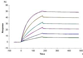
Biotinylated Human CD20 VLP captured on CM5 Chip via streptavidin can bind Rituximab, hFc Tag with an affinity constant of 0.40 nM as determined in SPR assay (Biacore T200).
